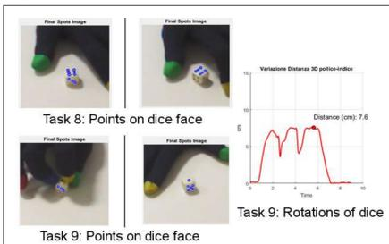
Detection of points on dice face to evaluate rotation of dice for Task 8 and 9 of MESUPES-Hand
