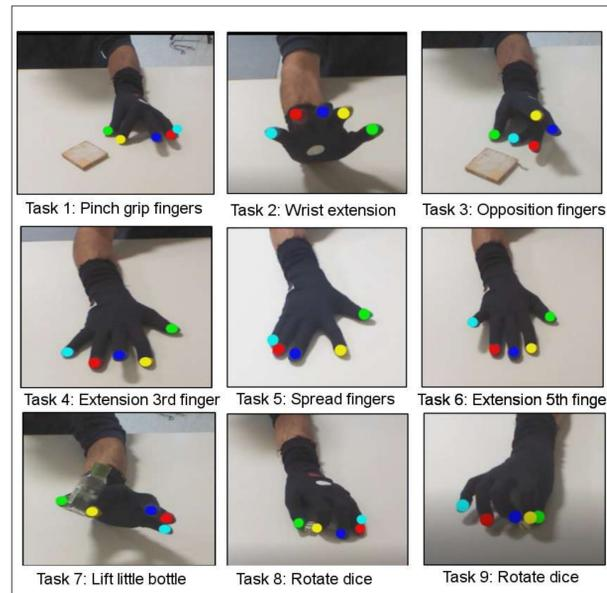
Tracking of hand and fingers movement while performing the motor tasks of MESUPES-Hand
