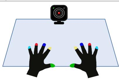
Setup of Hand Tracking acquisition system: hands on table, gloves with colored markers, RGB-Depth sensor to capture hand and fingers movement.
