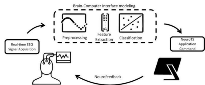
Block diagram of closed loop BCI procedure.
