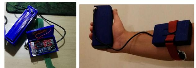
Fig. 3. (a) The proposed prototypal wearable device; (b) the realized device worn by a patient.
