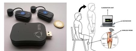
Fig. 2. (a) EMG FREEEMG1000 acquisition system; (b) Sit To Stand test setup.
