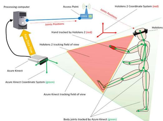
Fig. 1. Schematic representation of the setup proposed, combining Azure Kinect and Hololens 2.
